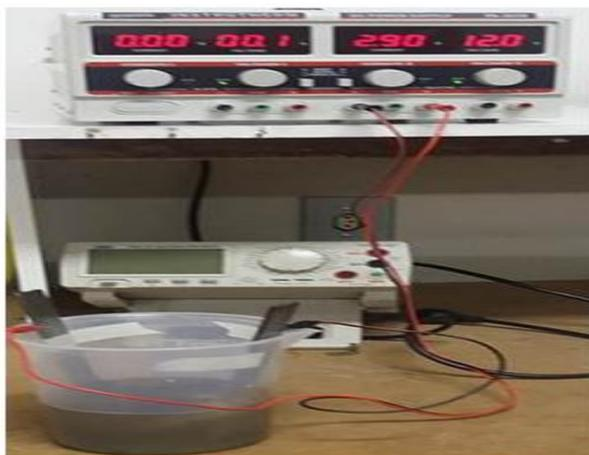
**Figure 1** – Assembled electrochemical reactor for electroflocculation of wastewater from biodiesel purification process
